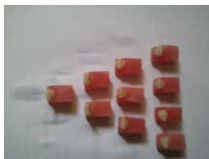
Fig. 1H. Specimens after finishing and polishing.
