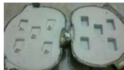
Fig. 1F. Group 2 after flasking in stone.
