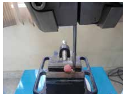
Fig. 2. specimen with chucks in place ready for testing
